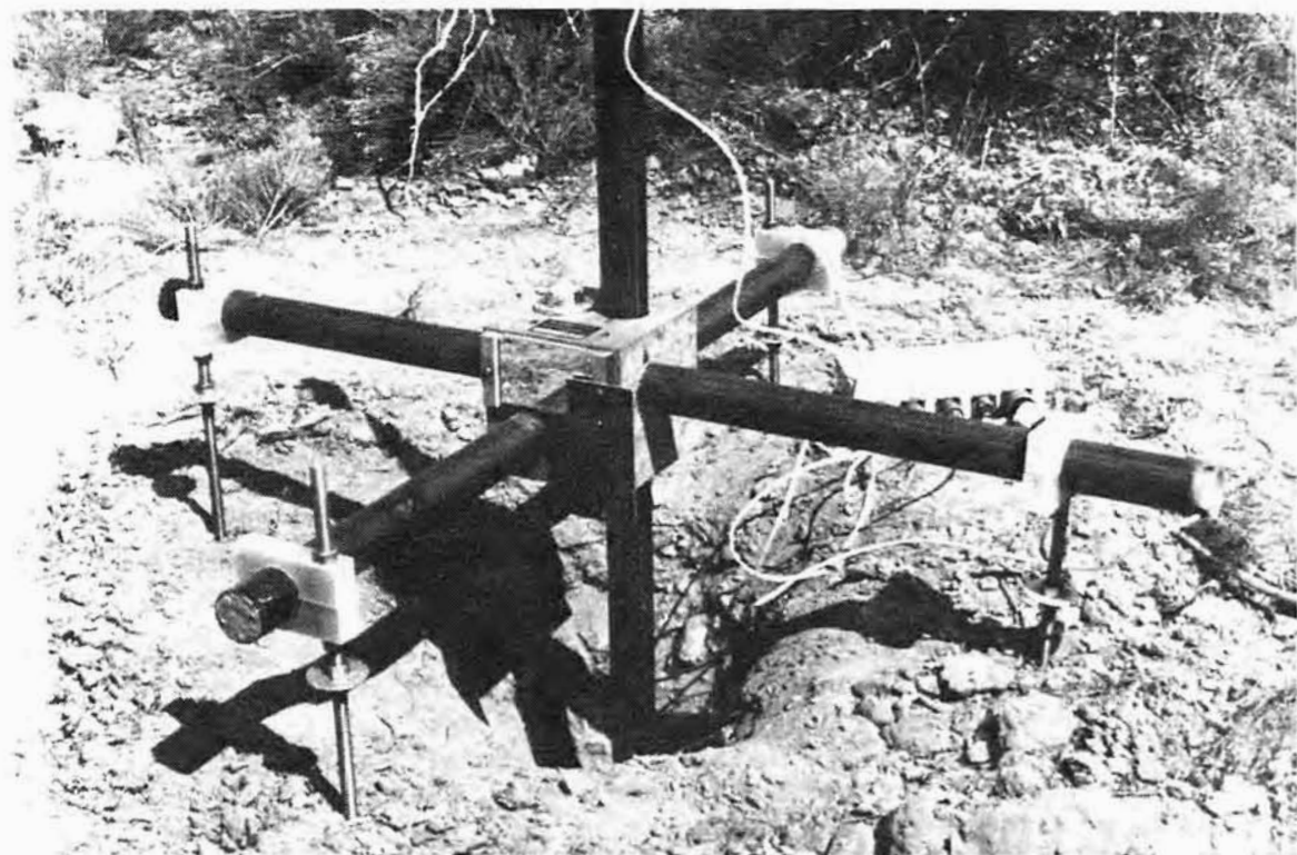
FIGURE 5-2. Three-axis search coil surface sensor measures signals from transmitter-loop in mine.
