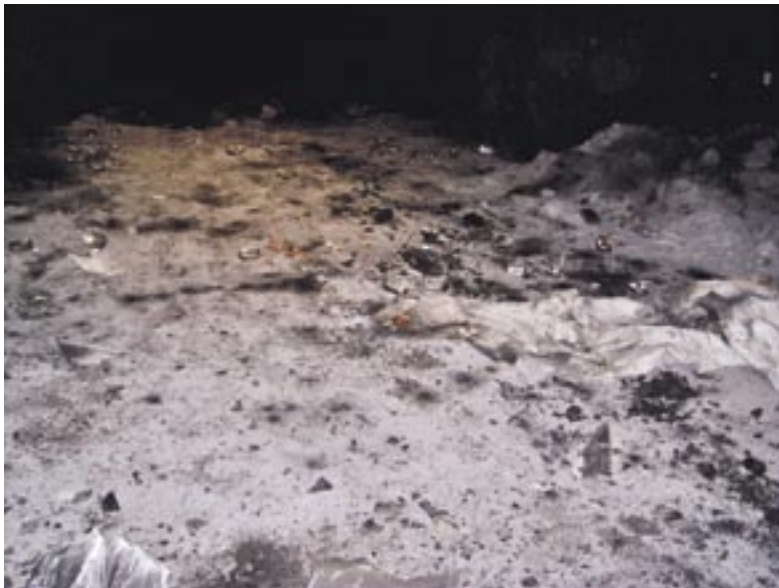
Discarded pieces of the 2 nd Left crews SCSR's were found in the #7 entry at about the eleven block. The picture indicates all the miners donned their rescuers at the same time at this location.
