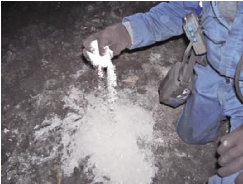
The forces of the explosion completely destroyed the Omega Block seal. Fine powder and dust was all that remained of most of the seal material.
