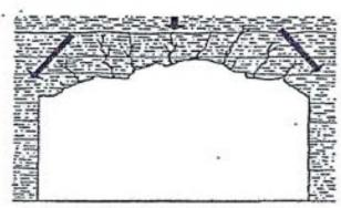
Vertical load is transferred to pillars as roof works its way into an arch.
