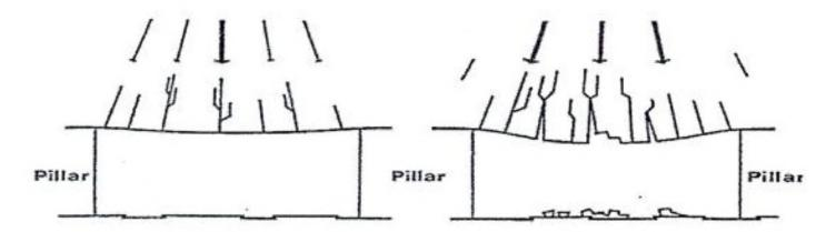
In the first stage, the roof begins to <u>sag</u> and tension cracks appear The center of the roof breaks, wedging itself, and the vertical load increases
