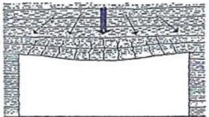
In early stages, the roof begins to sag, then tension cracks begin to appear.
