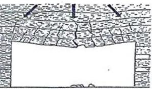
Roof center breaks, wedges itself, and the vertical load greatly increases.
