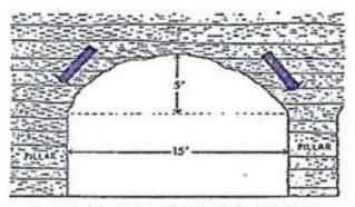
Roof has completely fell and forces are transmitted to pillars. Falling may; take minutes, days or even months.
