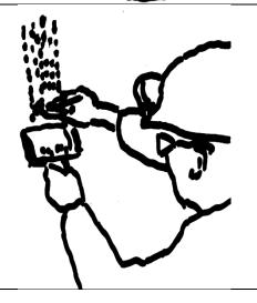
Rib/Roof Step 3 – Starting at the point of the rib where the floor sample ended, use the brush to gently remove one-eighth inch (1/8") of dust from the rib to the point where the vertical four inch (4") line reaches the roof. (If Rib/Roof appears too wet go to Wet Sampling Procedures below) Take care to prevent air currents from blowing the dust away while sampling by placing yourself upwind. The result should be a continuous vertical four inch (4") line from floor to roof.
