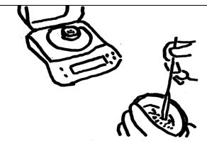
TGA Step 4 – Scan the porcelain crucible's barcode place it on the scale and add approximately 0.5 grams of the sample pressing the print button to enter the data into the database.
