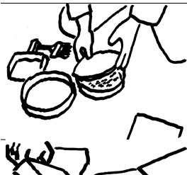
Rib/Roof Step 9 – Remove the sieve section and discard the oversized material. Place the lid on the pan and shake gently to ensure the contents are adequately mixed.
