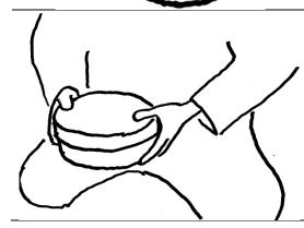
Rib/Roof Step 8 –With the collected material from each rib and the roof now placed into the sieve with the pan section below and the lid on shake gently. Use a rocking motion always keeping the lid upright. Check periodically until all the material capable has passed through the sieve.
