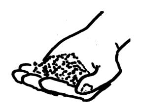
Wet Step 1 – If it is suspected that either the floor or rib/roof sampling location may be too wet use the rubber trowel to remove enough material to make a dust ball in the palm of the hand from the top one-eighth inch (1/8"). If when squeezed reasonably in a hand liquid flows with between fingers leaving a wet residue in the hand it can be concluded that the dust may be too wet. Visual observation is not sufficient for determining too wet.
