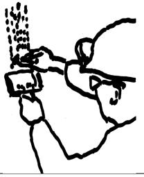
Rib/Roof Step 1 – Starting at the point of the rib where the floor sample ended, use the brush to gently remove one-eighth inch (1/8") of dust from the rib to the point where the vertical four inch (4") line reaches the roof. (If Rib/Roof appears too wet go to Wet Sampling Procedures below) Take care to prevent air currents from blowing the dust away while sampling by placing yourself upwind. The result should be a continuous vertical four inch (4") line from floor to roof.
