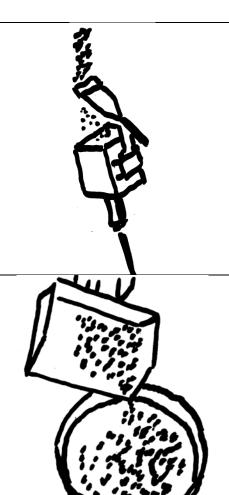
Rib/Roof Step 1a – If the rib is too high to reach the roof utilize the rib brush adapter for the scoop and an extension rod. Starting at the point that could be reached without an extension, place the brush with the adapter against the rib and raise upward to where the rib meets the roof collecting the surface one-eighth inch (1/8") of dust. Care should be taken to ensure the scoop does not scrape the rib. The result should be a continuous vertical four inch (4") line from floor to roof.
