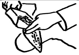
Floor Step 4 – Ensure that scoop is free of any material then transfer the mixed sample back to the scoop taking care to prevent air currents from blowing the dust away. Using the scoop, pour approximately an eight ounce (8 oz) volume into the sample bag and seal – this is approximately the amount that will fit in small coffee cup. If there is insufficient sample repeat the procedure creating another sampling line immediately adjacent to the first. Any excess can be discarded.
