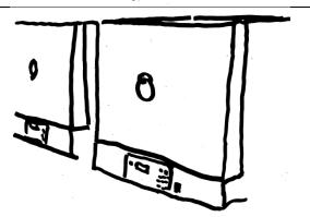
TGA Step 9 - Place the batch of crucibles in a Muffle Oven programmed for a 90 minute ramp up to 515°C then hold for 150 minutes.
