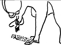
Floor Step 1 – Starting at the point where the rib meets the floor on one side of the sampling location use the brush and the scoop to gently remove the top one-eighth inch (1/8") in a strip approximately four inches (4") wide at right angle to the rib until you reach the opposite rib. As ripples in the floor are encountered be careful to not over sample the ridges or troughs. (If floor appears too wet go to Wet Sampling Procedures below)
