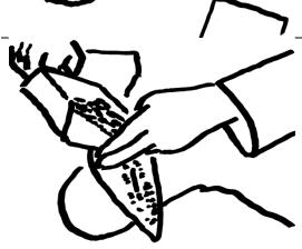
Rib/Roof Step 10 – Transfer the material back to the scoop then pour approximately an eight ounce (8 oz) volume into the sample bag. This is approximately the amount that will fit in small coffee cup. Any excess can be discarded. If there is insufficient sample repeat the entire rib/roof procedure creating another sampling line immediately adjacent to the first.
