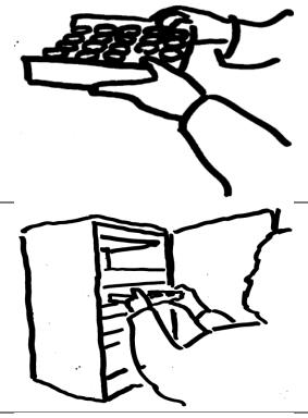
TGA Step 6 - Place weighted crucibles in a tray and place the tray in a drying oven, set to 105°C for a period of one hour.
