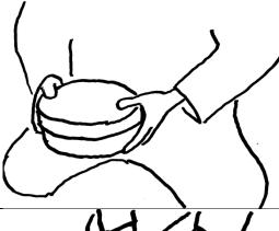
Floor Step 2 – Place the materials collected into the sieve with the pan section below and the lid on and shake gently. Use a rocking motion always keeping the lid upright. Check periodically until all the material capable has passed through the sieve.
