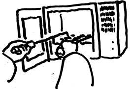
TGA Step 8 - Place the tray of samples in a desiccant holding cabinet until a full batch of samples is ready to place in the Muffle Furnace.
