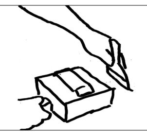
Starting at the point where the rib meets the floor on one side of the sampling location use the rubber sampling tool and the scoop to gently remove the top one-eighth inch (1/8") in a strip approximately four inches (4") wide at right angle to the rib until you reach the opposite rib. As ripples in the floor are encountered be careful to not over sample the ridges or troughs.
