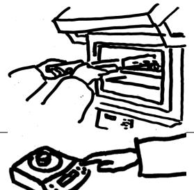
TGA Step 10 – Allow to muffle oven to cool to approximately 100°C then remove the trays using the rods to avoid burns. Place the tray into the desiccant holding cabinet until cool enough to handle.
