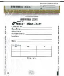
Step 7 – No sieving is required for wet samples, the sample bag should be sealed once the entire sample has been collected.
