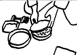
Floor Step 3 – Remove the sieve section and discard the oversized material. Place the lid on the pan and shake gently to ensure the contents are adequately mixed.
