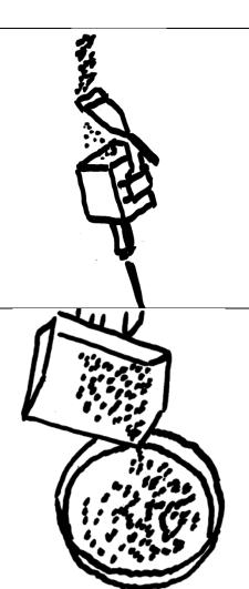
Rib/Roof Step 3a – If the rib is too high to reach the roof utilize the rib brush adapter for the scoop and an extension rod. Starting at the point that could be reached without an extension, place the brush with the adapter against the rib and raise upward to where the rib meets the roof collecting the surface one-eighth inch (1/8") of dust. Care should be taken to ensure the scoop does not scrape the rib. The result should be a continuous vertical four inch (4") line from floor to roof.
