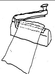
TGA Step 5 - Place the remainder of the sample in the original sample bag and place that in a clear poly sleeve such that the labels and notes can be seen without opening. Use the impulse sealer to secure the bag, transferring it to the evidence room after the batch is processed.
