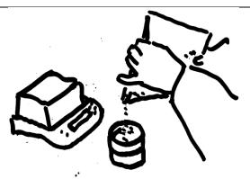
TGA Step 2 – Cut the bag with scissors above the barcode without completely removing the top of the bag. Prepare sample for analysis by passing through a US Standard No. 20 sieve. In sieving, the entire sample should be shaken until it is evident that no more of the course particles will pass through into the pan beneath.
