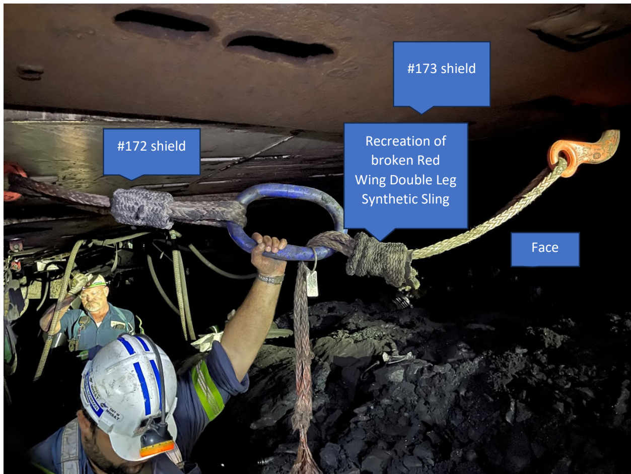
Photo of the accident scene at 10 Left Longwall Face.
