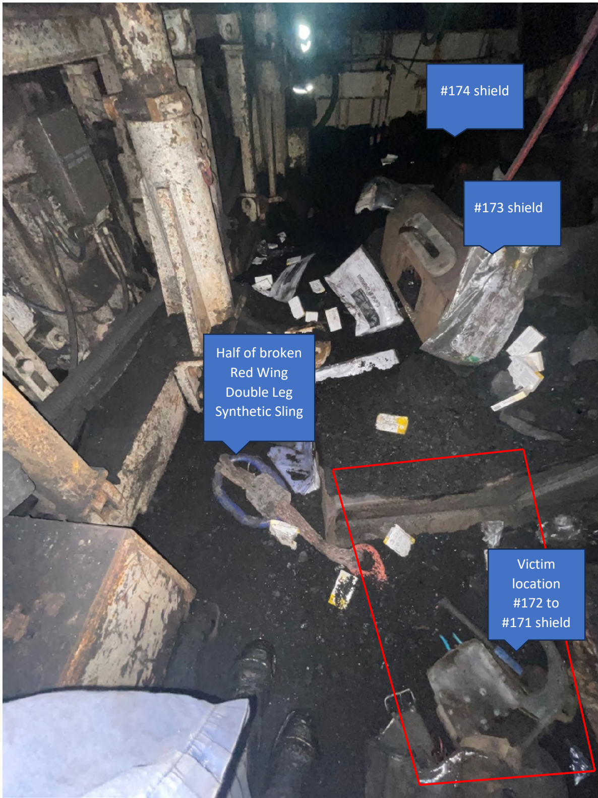
Photo of the accident scene at 10 Left Longwall Face.
