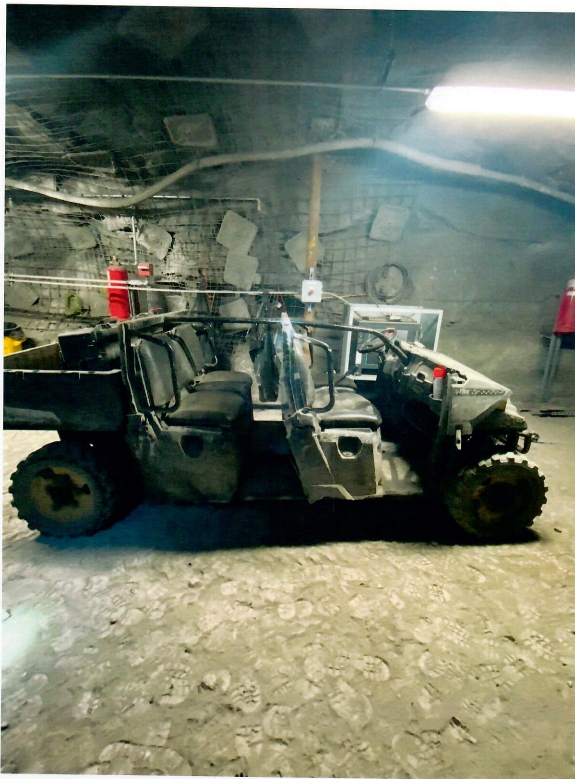
The purpose of this photo is to depict what a typical 4 man Electric Mining Utility Vehicle (“EMU”) would look like. This is identical to the EMU involved in the accident.
