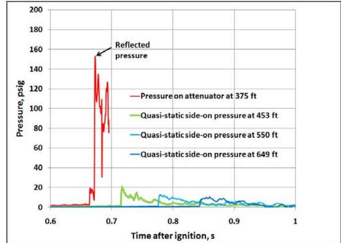
**Figure 12.** Reflected explosion pressure inby the Attenuator and the quasi-static pressure 78, 175, 274 and 432 ft outby the Attenuator during the second test (LLEM Test #526).
