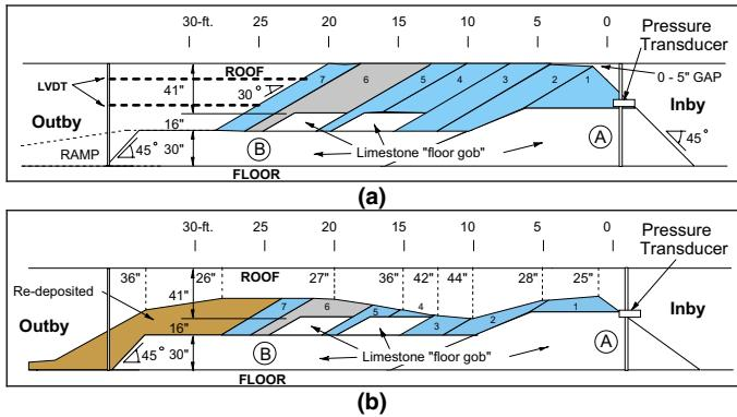
**Figure 7.** Configuration of Mine Blast Attenuator before (a) and after (b) the first test (LLEM Test #525). White: 46-cm (18-in.) x 0 limestone rubble, Blue: 15-cm (6-in.) x 0 crusher-run limestone, Gray: Mixed 15-cm (6-in.) x 0 and Limestone, Brown: Re-deposited material (undifferentiated).
