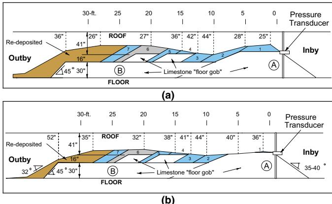
**Figure 10.** Configuration of Mine Blast Attenuator before (a) and after (b) the second test (LLEM Test #526).
