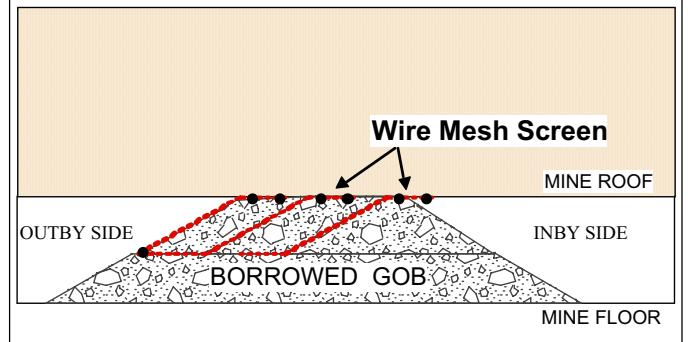
**Figure 2.** The "fully-stowed" alternate Attenuator design with sections of corrosion resistant wire mesh to provide confinement and passive reinforcement to minimize material erosion during the pressure blow down. This design was tested and evaluated in full-scale explosion tests at the NIOSH Lake Lynn Experimental Mine, but without the wire mesh screen.
