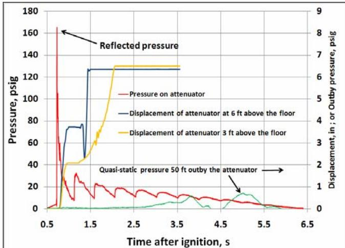
**Figure 9.** Reflected explosion pressure inby the Attenuator (A-375) and the quasi-static pressure 15 m (50 ft) outby the Attenuator (A-453) during the first test (LLEM Test #525). Displacement of the Attenuator as measured with LVDTs is also shown.
