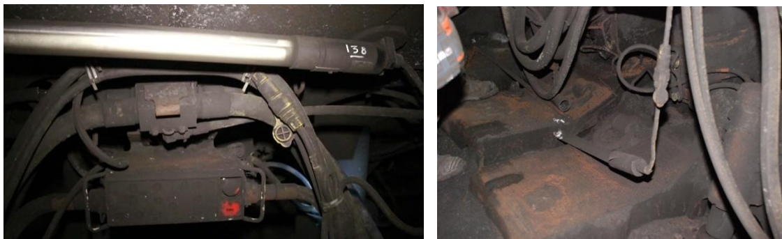
Figure 12. (LEFT) Fluorescent light hanging intact at Shield 138. (RIGHT) Fluorescent light, partially intact, but pulled off its mounts and down at Shield 74
