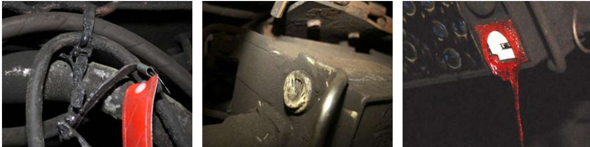
Figure 1. (LEFT): Melted zip ties; Shield 38; (MIDDLE): Melted speaker cover; Shield 39; (RIGHT): Melted plastic lens cover on Shield 62 control box (CIU). Note the clean white area behind the melted red lens.
