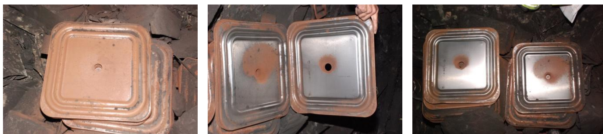
Figure 11. A stack of square pans found near the mouth of #22 Headgate survived the explosion and exhibited general rusting on their outside surfaces. Inside the stack, the only rusting was in the vicinity of the 1" roof bolt hole. It is believed that the "patina rusting" is due mainly to heat vaporizing some or all of the galvanized finish. Abrasion by wind-born particles may also play a role.
