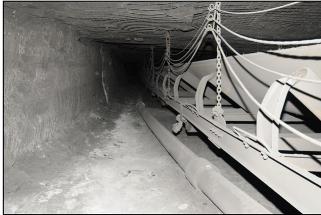
Figure 1A. Between crosscuts the belt structures are relatively intact. This is an example view of a suspended belt structure near spad 19819, North Glory Mains (NGM), looking inby.
