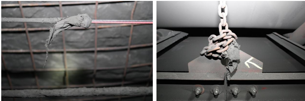
Figure 18. (LEFT) North Glory Mains: 50-ft SE of spad 20045 (SW view). The heated outer insulation of the phone line is bunched in the direction of Final Forces, which were directed SE. (Note: The original photograph was taken from the opposite side of the belt. It has been inverted here to a comparable SW view).
