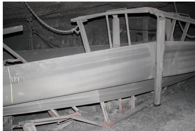
Figure 1B. In crosscuts, explosion forces entering perpendicular to the belt and from the SW side cause a CCW rotation of the belt structure, which would be from the LEFT side, looking inby (left lateral). This example view is near spad 19835 in NGM, looking to the SW from the edge of the crosscut.
