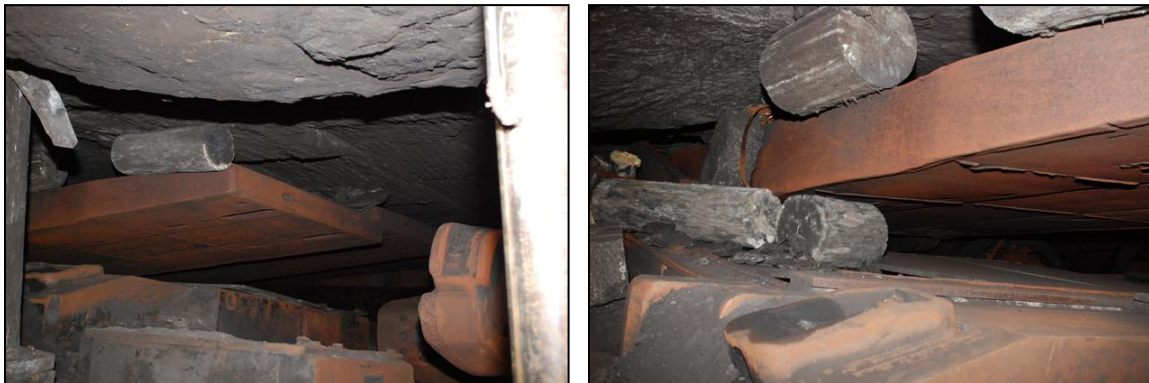
Figure 10. (LEFT): Short lengths of support posts were carried by winds entering the tailgate, traveling north, and impacted between the roof and top of Shield 176. This is a view from the tailgate, looking NW. (RIGHT): Any subsequent winds from the north were not sufficient to blow these back down.
