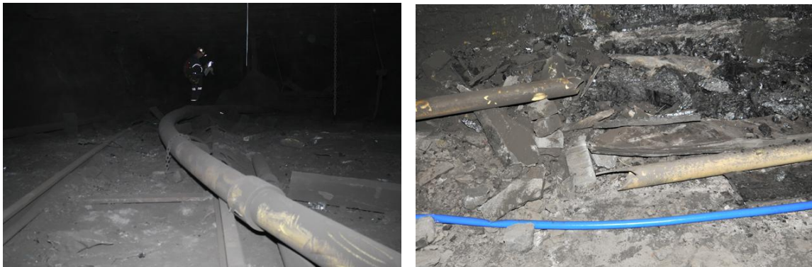
Figure 8. (LEFT) Example of a waterline moved by explosion forces. (RIGHT) An example of a small waterline broken (perhaps by explosion forces).
