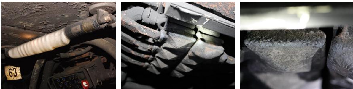
Figure 2. (LEFT): Melted fluorescent light cover at Shield 62; (MIDDLE): Evidence of heat on the rubber cover for manual shield control box; Shield 62; (RIGHT): Close-up of cover for manual shield control box; Shield 62.
