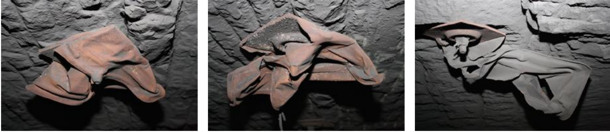
Figure 7. Examples of severe roof pan damage in the region of #21 Tailgate south of the the #21 Cross-over.
