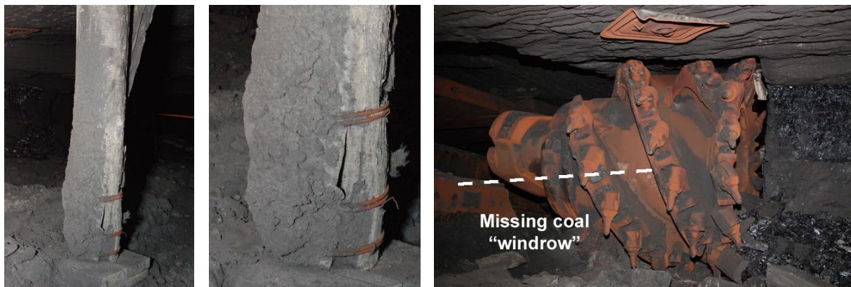
Figure 5B. (LEFT): Impacted wet coal and dust along the bottom half of the first propsetter outby the shearer. This points toward the back (west) side of the shearer cutting head; (MIDDLE): Close-up view. (RIGHT): The coal “windrow” (coal berm) that normally develops here is missing.
