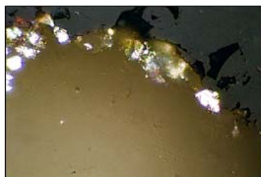
Collotelinite, quartz + pyrite
