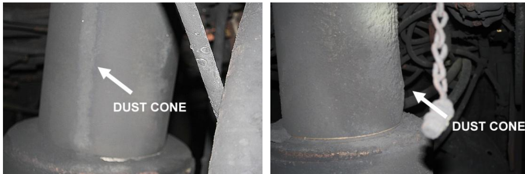
Figure 10. (LEFT) Cylinder leg on Longwall; South side of south jack, Shield 166. View looking NW. These are deposits are Final Forces features, originating from the Tailgate side of the longwall.
