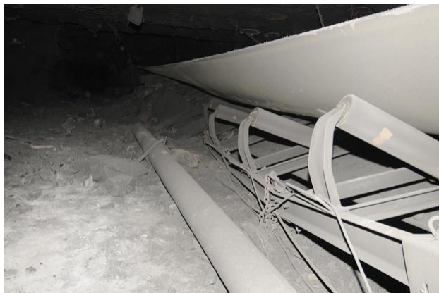
Figure 1C. After the CCW rotation the chain on the windward side may be broken, or the chain on the leeward side may become unhooked, dropping one side of the belt structure. This example view is in the North Glory Mains near spad 19852, looking inby.
