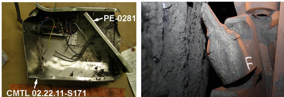
Figure 5A. (LEFT): Two pieces of the same Control box believed to have originated at Shield 173 (RIGHT): Impacted coal and dust along the north face of shearer bit, next to the solid coal face.
