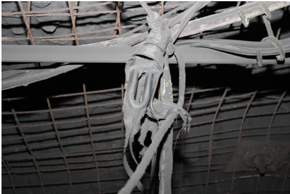
Figure 2. Undamaged lamp showing heat melting plastic cover on undamaged fluorescent lamp near longwall mother drive unit.
