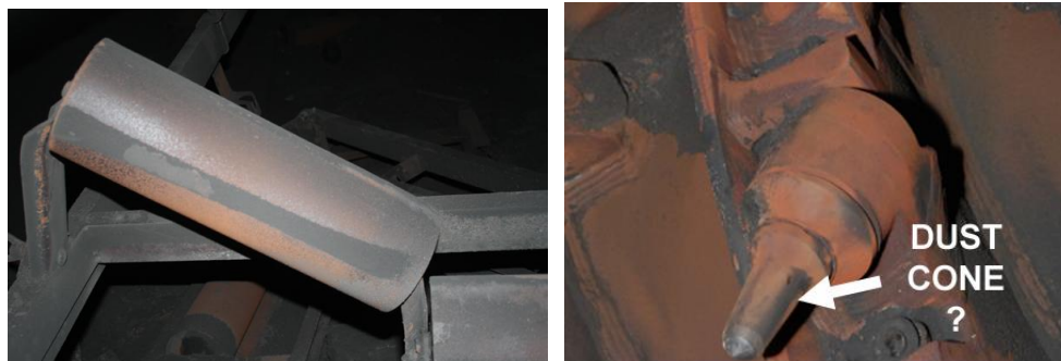
Figure 14. (LEFT) Roller on belt structure with impacted dust cone; #21 Cross-over, approximately 30 feet south of spad 23813, looking south. Final Forces were from the NORTH.
