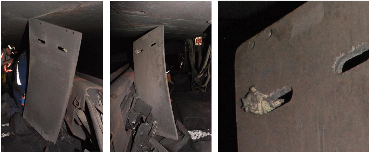
Figure 8. (LEFT): Aluminum cover off the tail-drive motor that came to rest in an upright position, wedged under the canopy at Shield 157 (view looking north). Because it was stopped this way the pressures responsible for its transport could not be calculated. (MIDDLE): South view, showing debris piled against north side. (RIGHT): South view, close-up of paper fragment caught in a grip hole.
