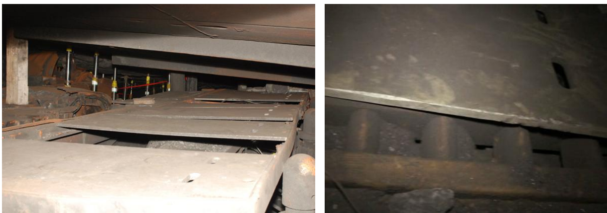
Figure 9. (LEFT): A view of the tail-drive; where two aluminum covers were removed by wind forces which came from the south. (RIGHT): One of the covers was found in the panline at Shield 130, having traveled approximately 256 feet.
