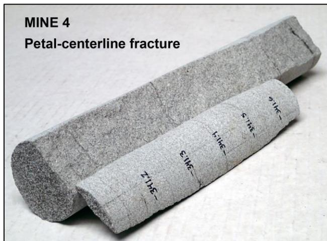
**Figure 15. MINE 4: One of three drilling-induced petal-centerline (P-C) fractures that corroborate the Diametral Method results are aligned with the inferred contemporary maximum horizontal stress direction.**
