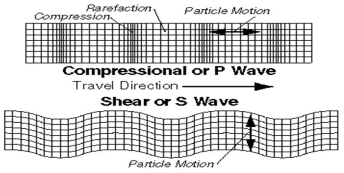
P waves shake the ground in the direction they are propagating, while S waves shake perpendicularly or **transverse** to the direction of propagation.
