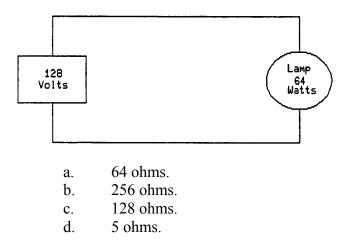
56. What is the voltage drop across the 64-ohm resistor?
