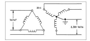
97. What is the turns ratio of the single-phase transformer shown below?
