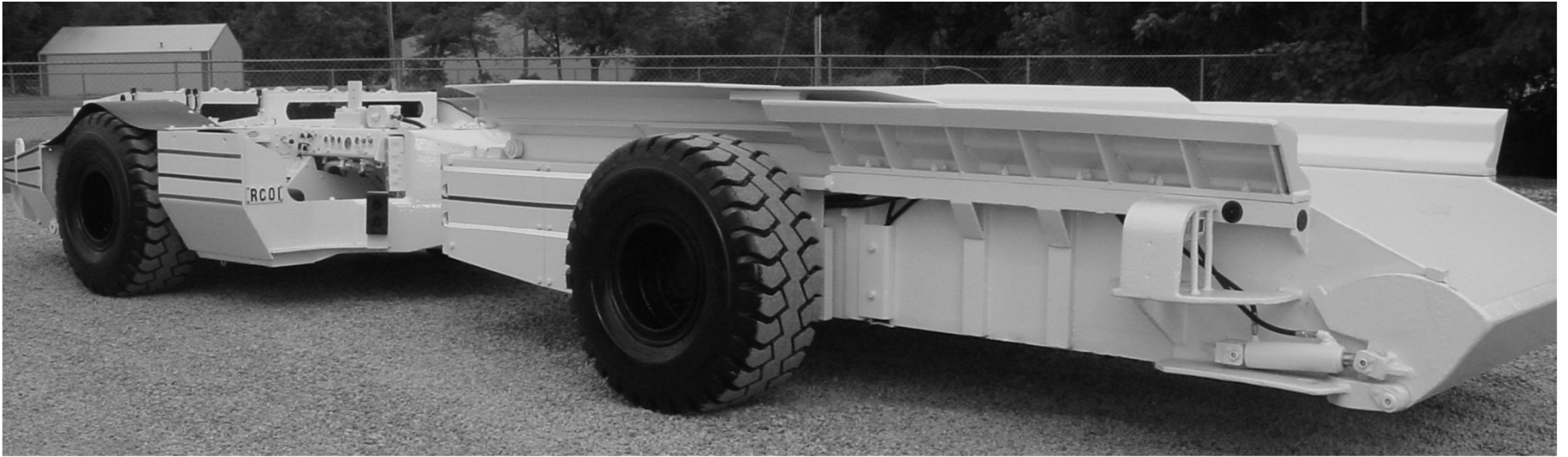
Jeffrey 4110 Ramcar re-powered and rebuilt by DST®
