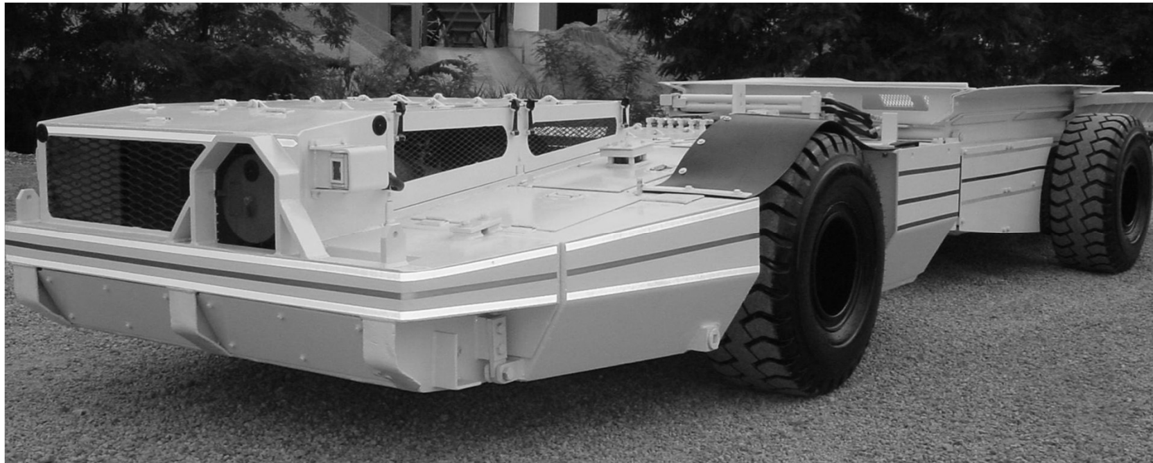
Jeffrey 4110 Ramcar re-powered and rebuilt by DST®
