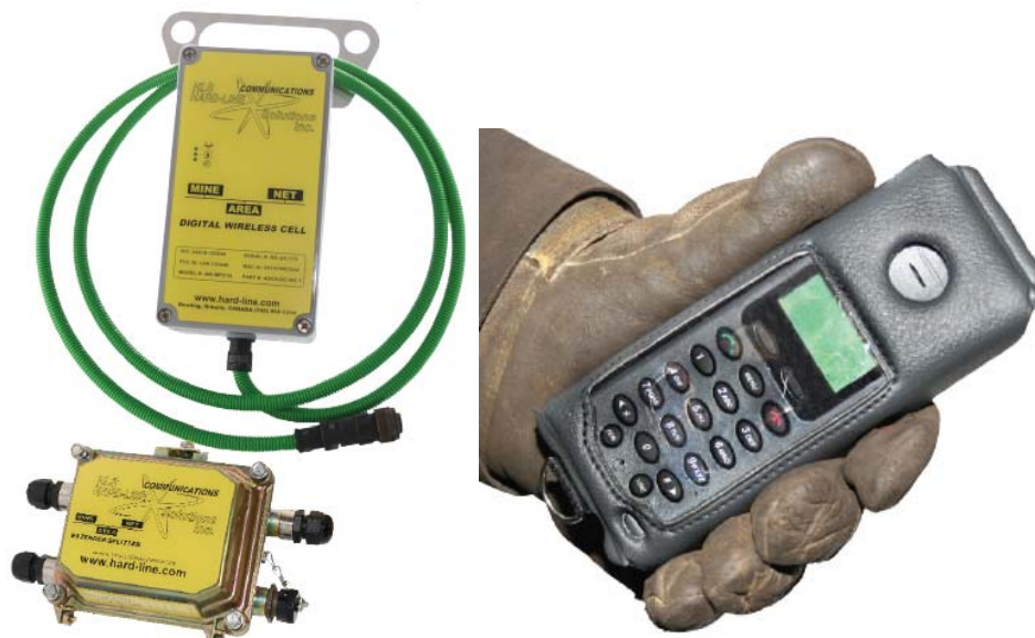
Figure 54 – Wi-Fi Access Point and VoIP Telephone from Hard-Line Solutions
