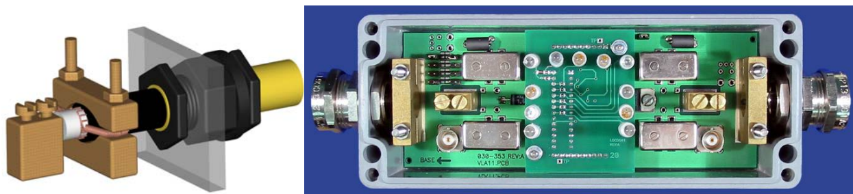
Figure 24 – Leaky Feeder Connection and Amplifier from MineCom
