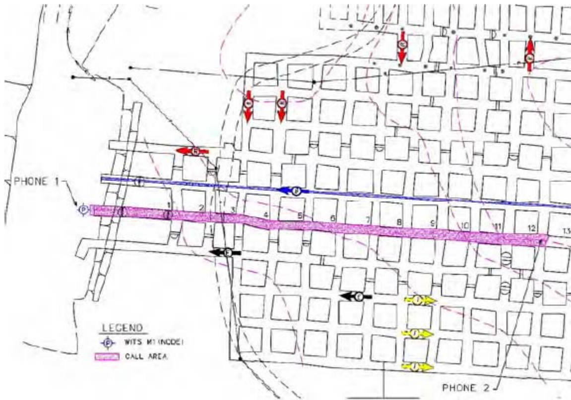
Figure 74 – Wi-Fi VoIP Telephone Communication over 900’ at the Tallmans Run #1 Mine Test Site
