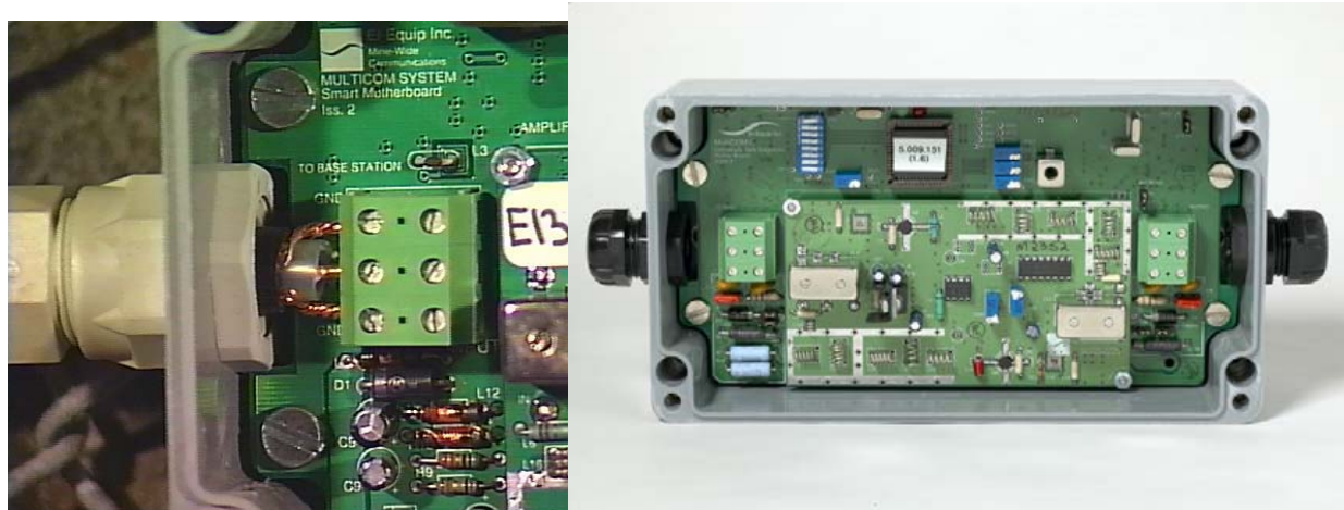
Figure 22 – MULTICOM Leaky Feeder Connection and Amplifier with Diagnostic Option from MRS
