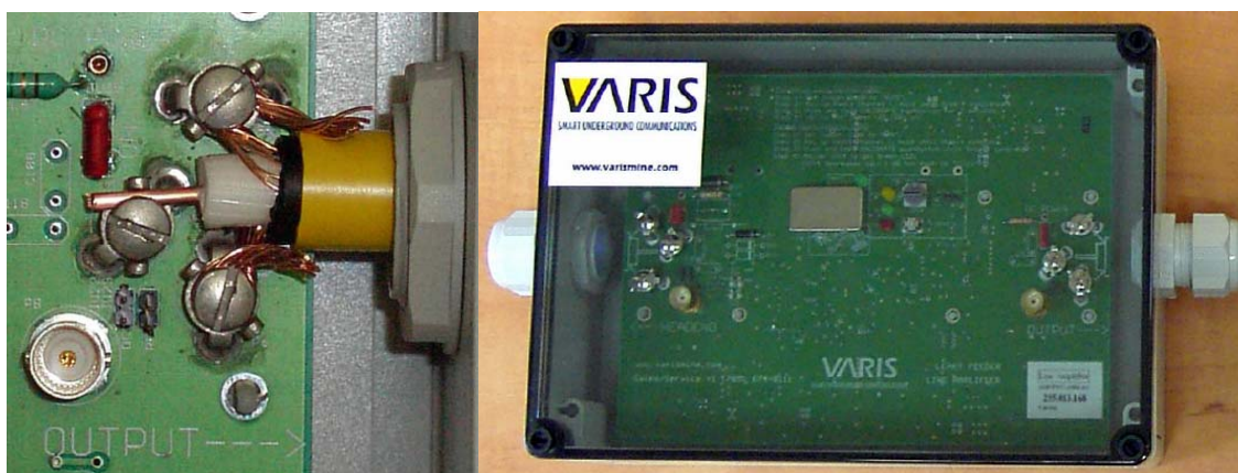
Figure 15 – Varis Leaky Feeder Connection and Amplifier
