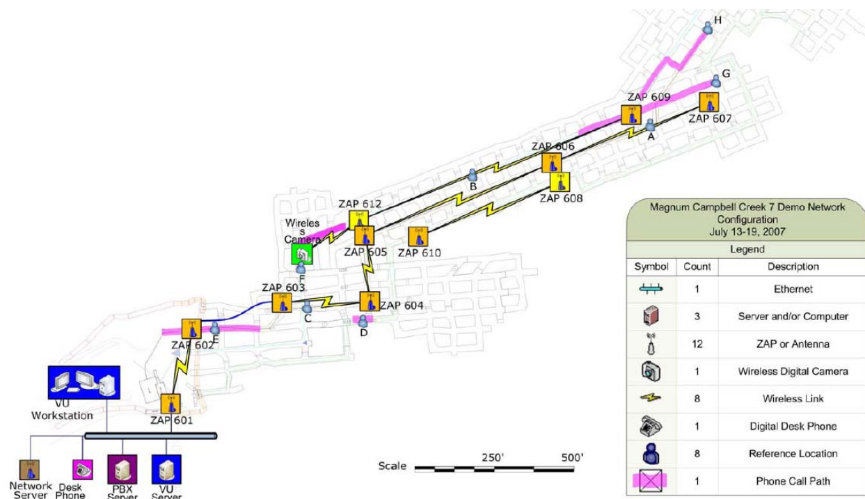
Figure 72 – Test Site at Campbells Creek #7 Mine
