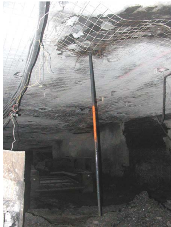
Photo 1: Sampling pipe through first borehole looking toward shuttle car across feeder in 23 crosscut
