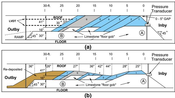
**Figure 7.** Configuration of Mine Blast Attenuator before (a) and after (b) the first test (LLEM Test #525). White: 46-cm (18-in.) x 0 limestone rubble, Blue: 15-cm (6-in.) x 0 crusher-run limestone, Gray: Mixed 15-cm (6-in.) x 0 and Limestone, Brown: Re-deposited material (undifferentiated).
