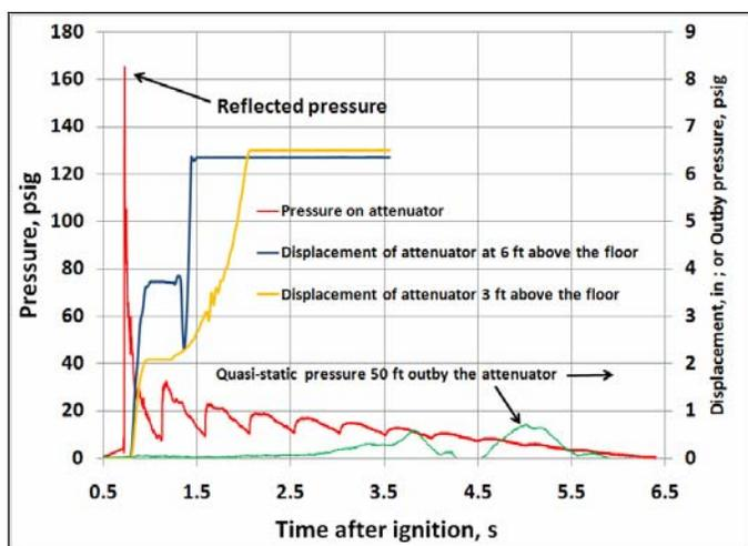
**Figure 9.** Reflected explosion pressure inby the Attenuator (A-375) and the quasi-static pressure 15 m (50 ft) outby the Attenuator (A-453) during the first test (LLEM Test #525). Displacement of the Attenuator as measured with LVDTs is also shown.
